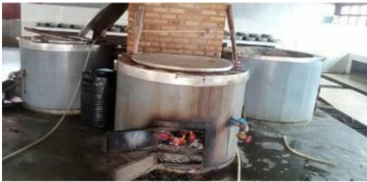
: Example of the Muvero cookstove that uses briquettes
