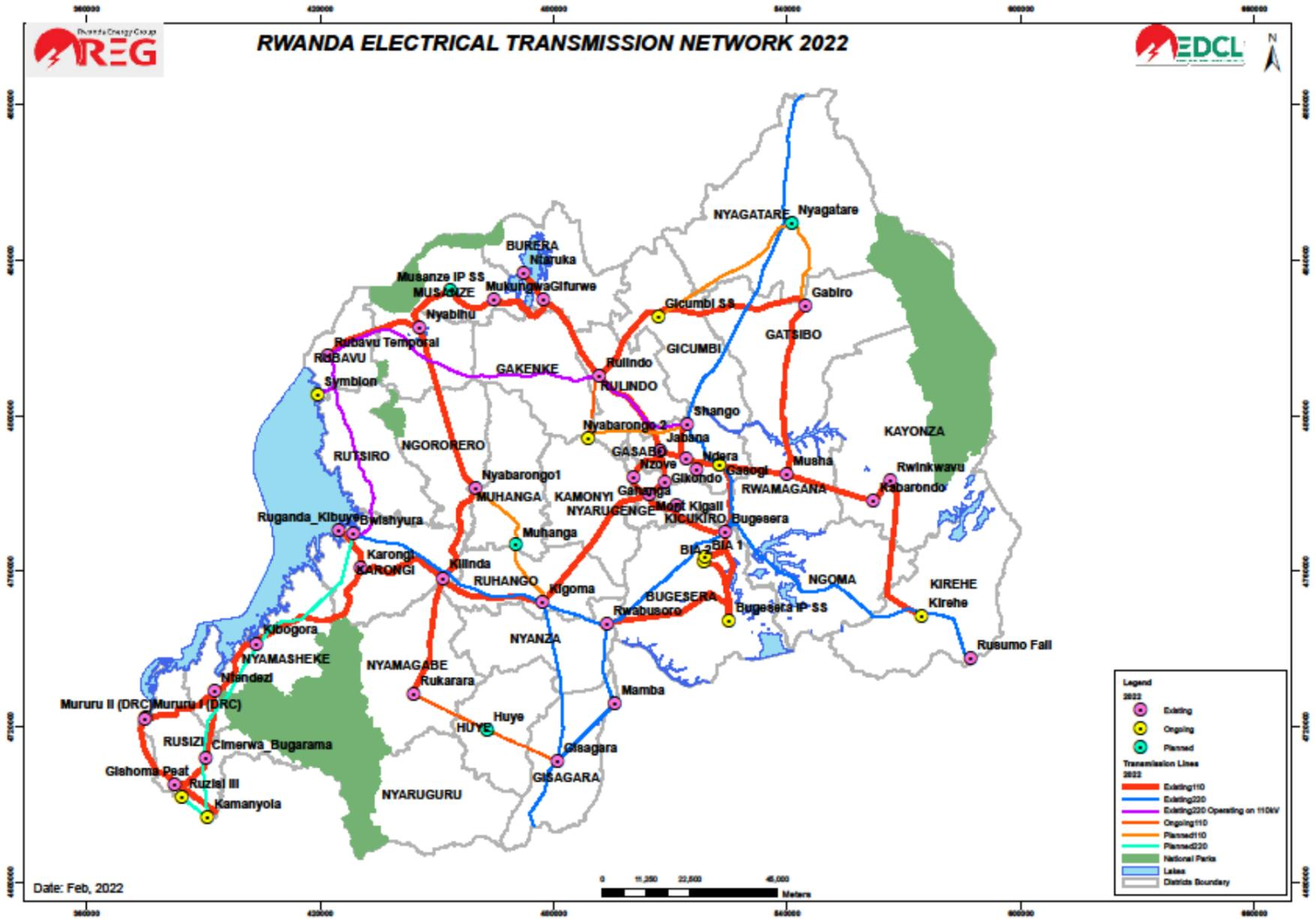
Figure 4: Transmission network (HV line) in 2022
