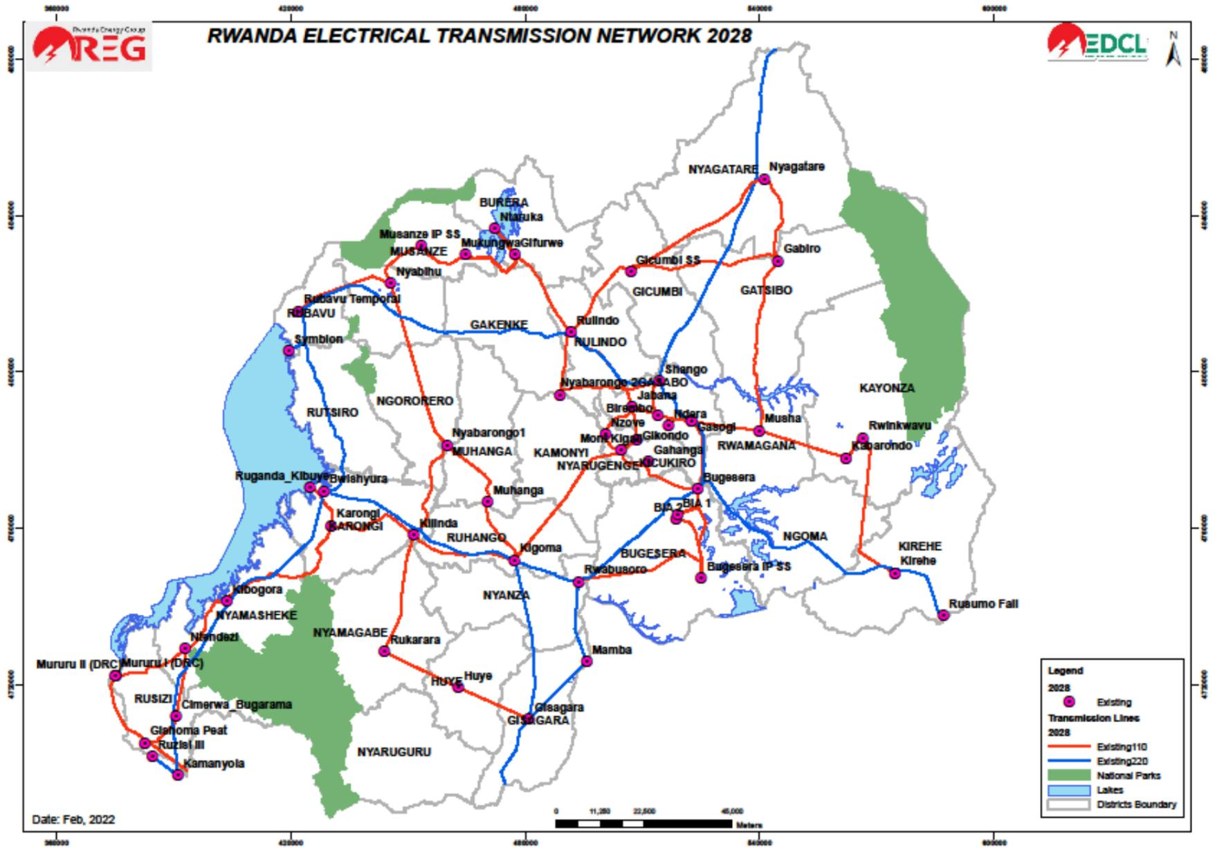
Figure 8: Transmission network (HV line) in 2028
