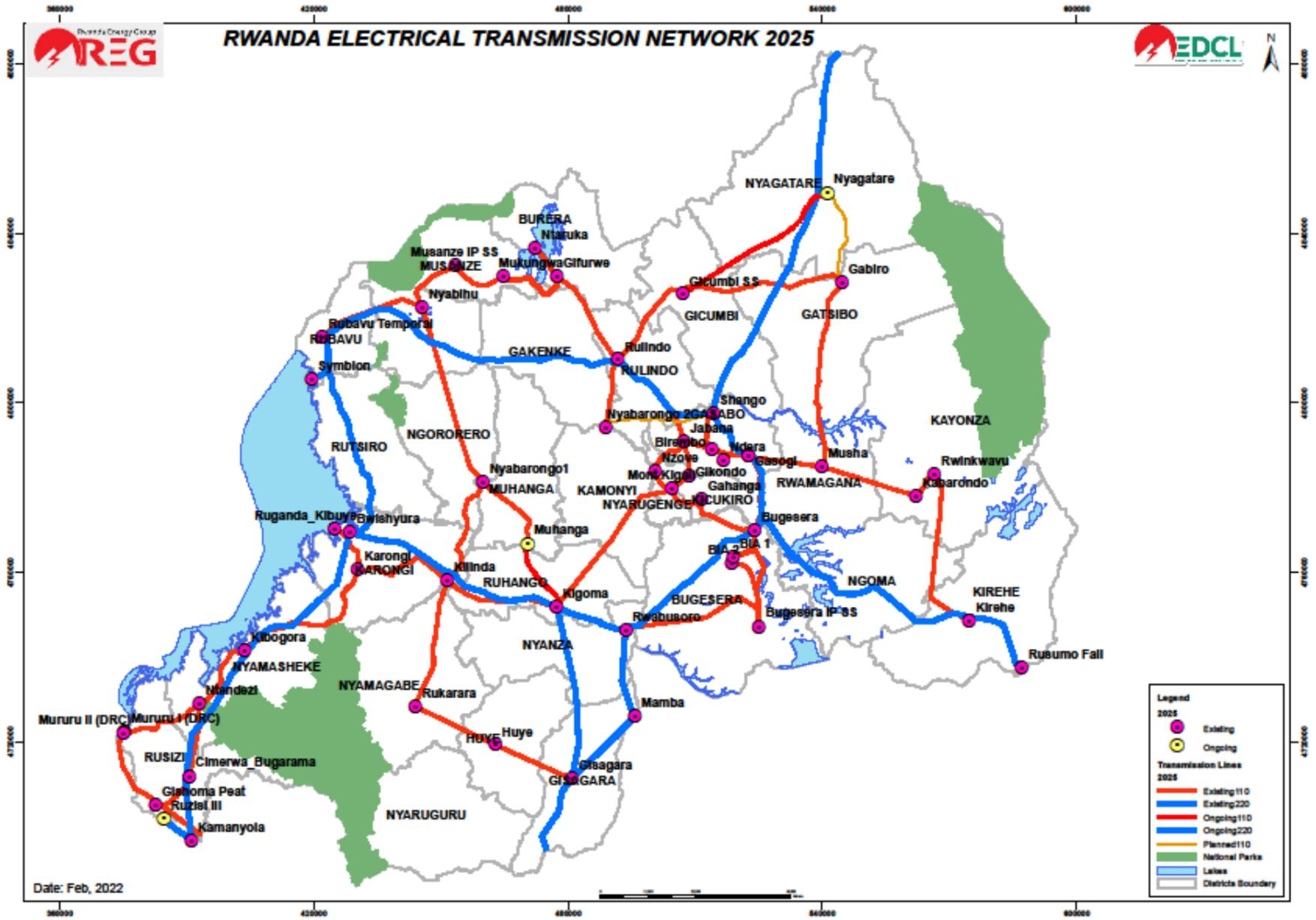
Figure 6: Transmission network (HV line) in 2025
