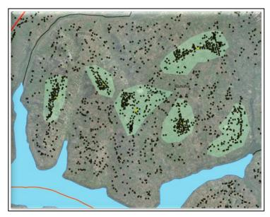
Figure 21: Population Clusters or 'Transformer Zones' Identified by Sofreco
