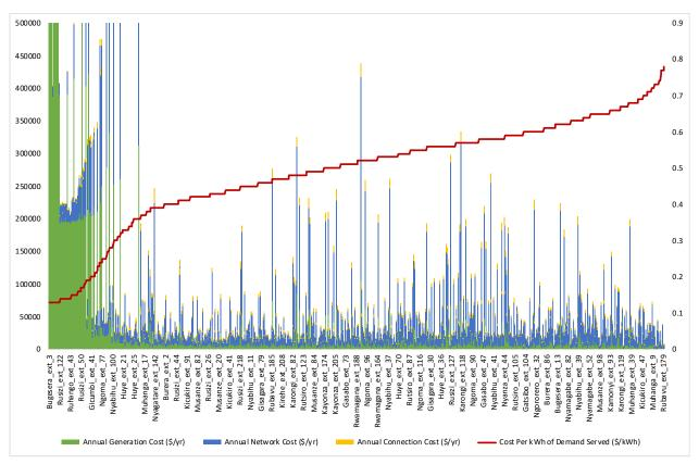
Figure 13 Breakdown of selected individual grid standard extension costs annuities (\$/yr) and per unit costs (\$/kWh). Rwandan National Electrification Plan – Reference Case Scenario
