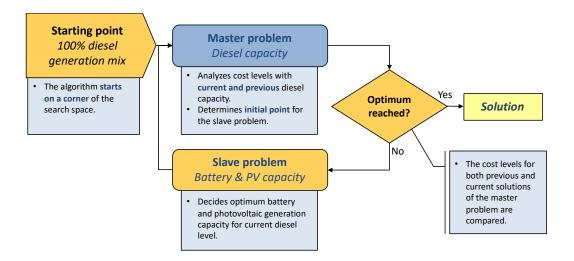
Figure 3: Master-Slave decomposition for the optimization of microgrid generation
