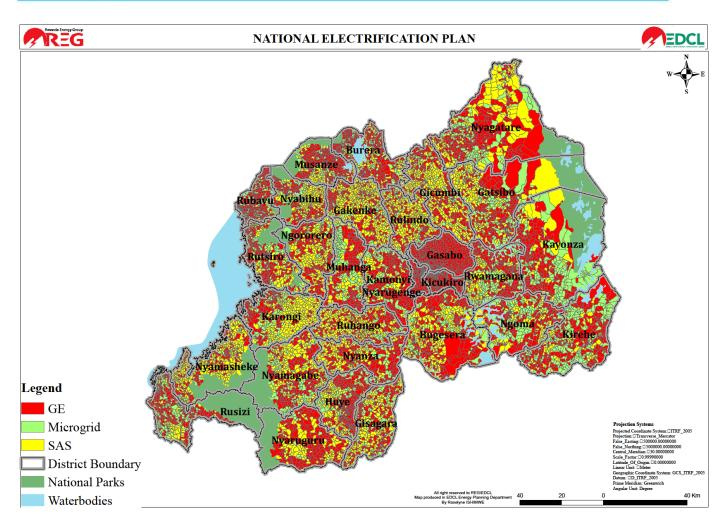
Figure 11 Systems map for the Rwandan National Electrification Plan – Reference Case Scenario
