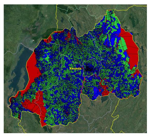
Figure 15 Satellite projection of grid extension villages (blue), off-grid villages (green) and High-Risk Zones (red) for the Reference Case Scenario
