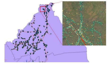
Figure 5: Sample image of different data sources: Sofreco (green dots), HRSL (yellow squares), MV (red lines) and LV (green lines) and 37.5 m buffer (light yellow) combined for the determination of location of non-electrified residential customers in Nyagatare district
