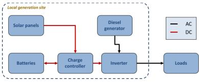
Figure 7: REM standard Microgrid Generation scheme
