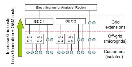
Figure 2: Example of structure of clusters (results from the clustering process)
