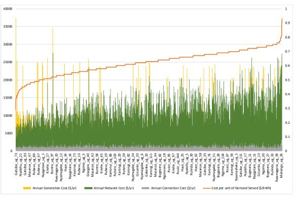
Figure 14 Breakdown of selected individual microgrids costs. Rwandan National Electrification Plan – Reference Case Scenario
