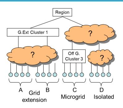
Figure 4: Example of minimum-cost electrification solution
