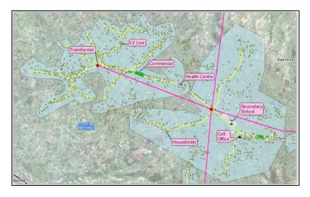
Figure 22: Illustration of Network Design for two Transformer Zones
